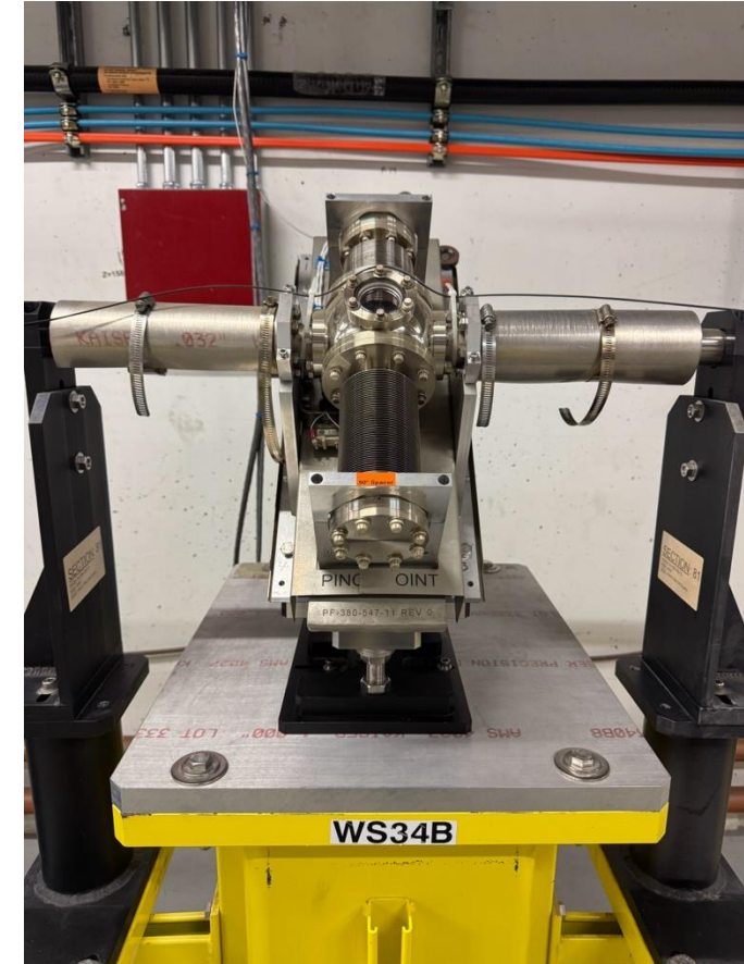
Fig.1: LCLS-II Wire Scanner in Undulator Hall
