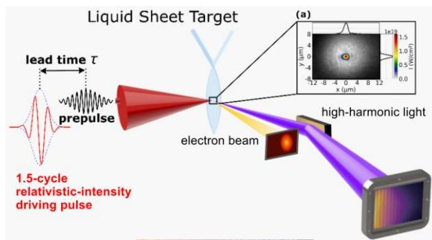
By employing flat ethylene glycol sheet targets with controlled plasma density gradients and relativistic-intensity, waveform-controlled near-single-cycle laser pulses, we have achieved reproducible high-flux RHHG with unprecedented stability [4]. Tuning of the driving laser waveform enables the generation of continuous XUV spectra, indicative of the isolated attosecond pulses [4].
