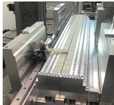
EU32: compact EPU for the APE-TX beamline
