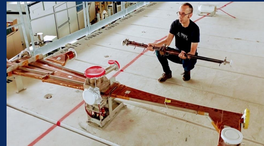
Dipole Arc Vacuum chamber SOLEIL/SOLEIL II
