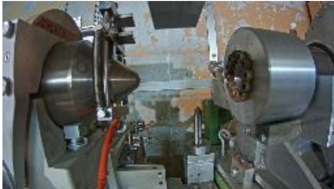
Temperature sensor installation on AD target
