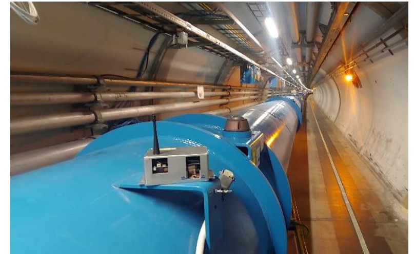
Radiation tolerant IoT hardware platform developed at CERN, courtesy of S. Danzeca
