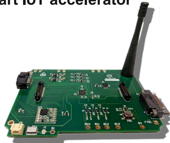
Radiation tolerant IoT hardware platform developed at CERN, courtesy of S. Danzeca
