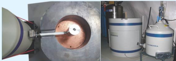
SAGeWell detector installed inside a lead castle
