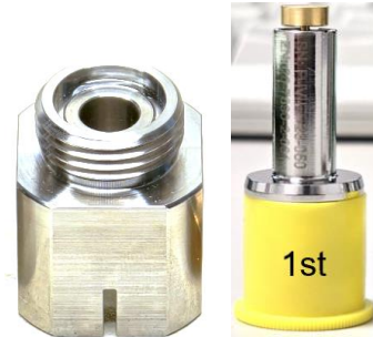
1 st batch of 30 feedthroughs in holder with adaptor
