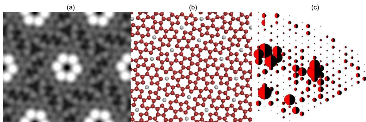
"Germanene" layer on Ag(111). a) STM image ( $6.0 \times 5.2 \text{ nm}^2$ ). b) corresponding atomic model (red: Ge atoms, grey: Ag atoms). c) comparison between experimental (red) and theoretical (black) in-plane structure factors.
