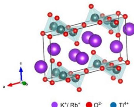
Figure 1 : Cristal structure of  $\text{M}_2\text{Ti}_2\text{O}_5$
