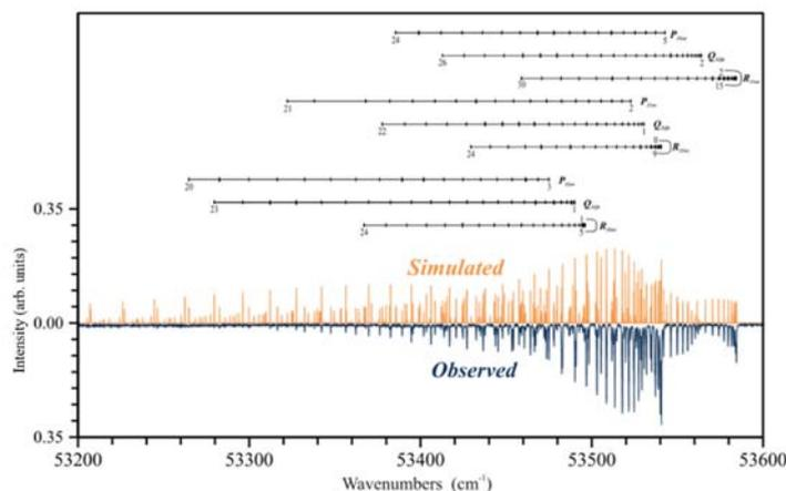
Fig. 1. Experimental spectrum of the  $^{12}\text{C}^{16}\text{O}$   $a^3\Pi - X^1\Sigma^+(3,0)$  recorded by VUV spectroscopy technique (lower, navy blue trace) as well as the simulated one plotted on the basis of the final deperturbation analysis using the PGOPHER software (upper, orange trace).
