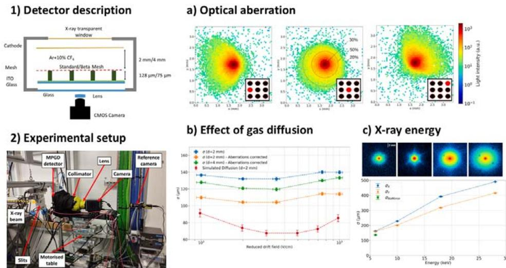
Figure 1: Schema of an optical readout detector and images from the experimental setup and different contributions to spatial resolution (optical aberration, gas diffusion and X-ray energy). Images published in [4].
