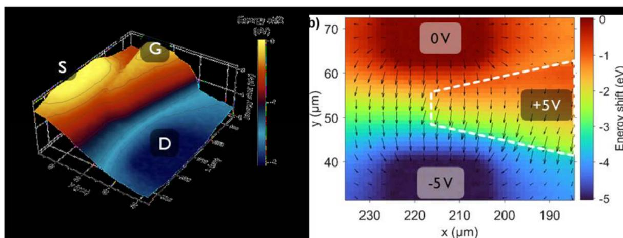
**Figure 1.** (a) Energy landscape of a back-gated field effect transistor ( $V_{DS}=-2$  V and  $V_{GS}=+5$ V). (b) Energy shift map (color map) and electric field map (arrow plot) in which the field direction and magnitude are given by the arrow for each position ( $V_{DS}=-5$  V and  $V_{GS}=+5$  V).
