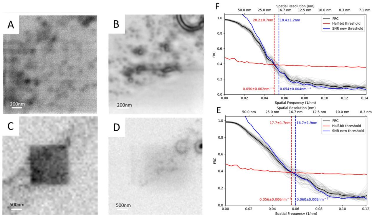
**Figure 1:** Intermixed NPs of PTQ10/ITIC-4F observed by STXM (A) and Ptychography (B). Images STXM (C) and (D) showed carbon deposition due to the precedent observation, STXM for (A) and Ptychography for (B) and graphics (E) and (F) correspond to FRC of image (A) and (B).
