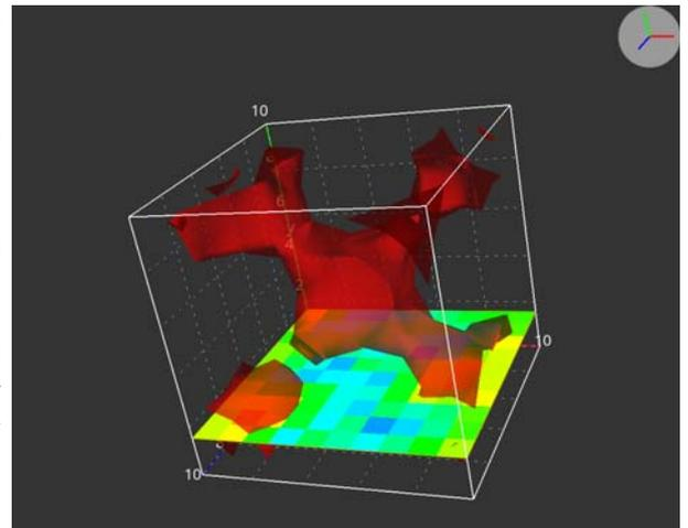
Figure 1:  $Mo_5PB_2$  electronic level isosurface in Brillouin zone.
