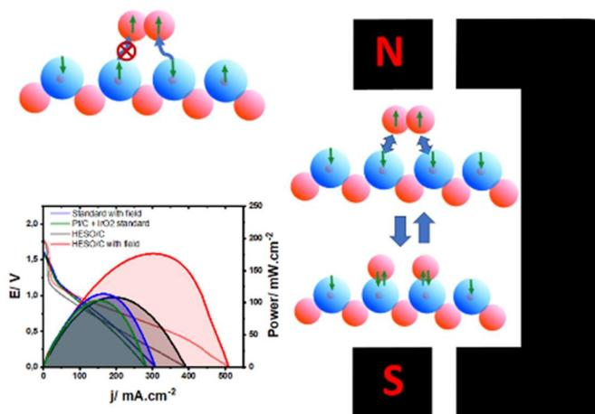
A high entropy spinel oxide  $(\text{CuCoFeMnNi})_3\text{O}_4$  was synthesized for use as a bifunctional oxygen evolution (OER) and reduction (ORR) reaction electrocatalyst for rechargeable zinc-air battery (RZAB) cathodes. An external magnetic field was used to induce enhancements in both the OER and ORR, as well as a dramatic improvement in the power profile of the zinc-air battery. This result is the most significant magnetic enhancement of a RZAB yet reported.
