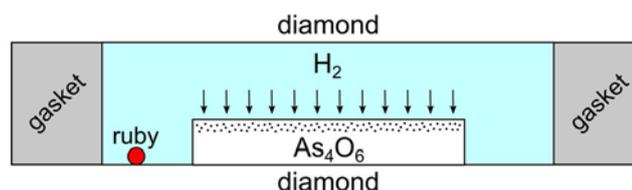
In addition to the reaction kinetics data, a method of growing thin plates of As<sub>4</sub>O<sub>6</sub> single crystals via spatial confinement will be presented. Using micro-sized thin-layered platelets (as shown in the Figure) proved to be a compelling way of studying the kinetics of diffusion in crystals. The measurements carried out at the SMIS infrared spectromicroscopy beamline in the SOLEIL Synchrotron clearly attest to the effectiveness of this new approach.
