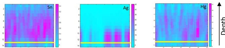
Fig. 3 – Depth elemental maps on the counterfeit *quattrino* of Lucca. The yellow line represents the surface of the coin. The tin map spans uniformly over the core of the coin, while silver and mercury are present only near the surface where the Ag+Hg layer was deposited, probably by dipping the coin in the amalgama.
